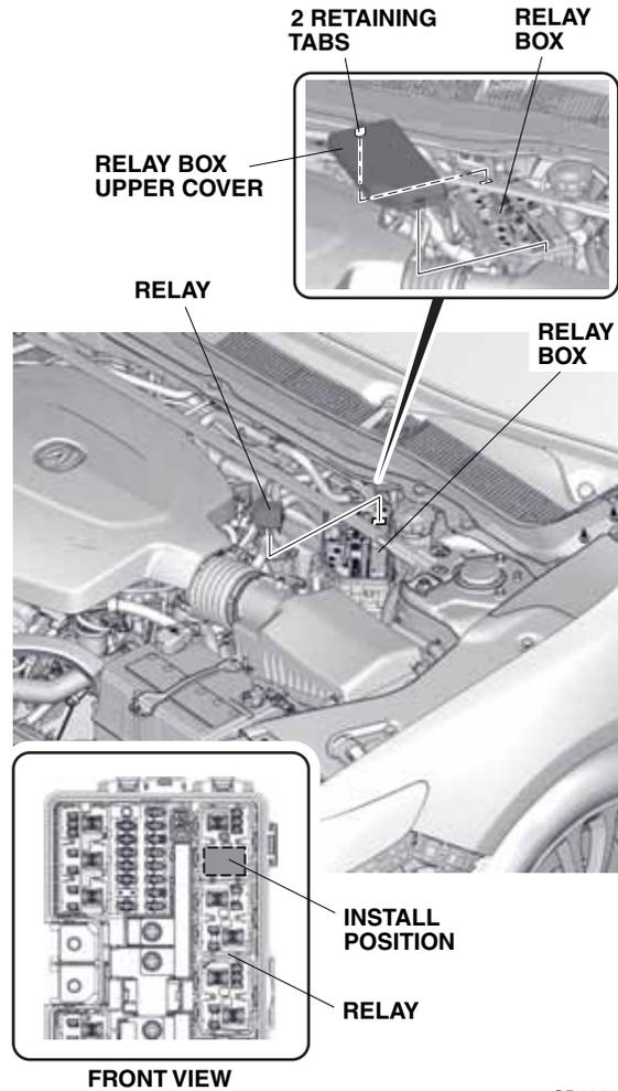
43. Install the relay into the relay box.
