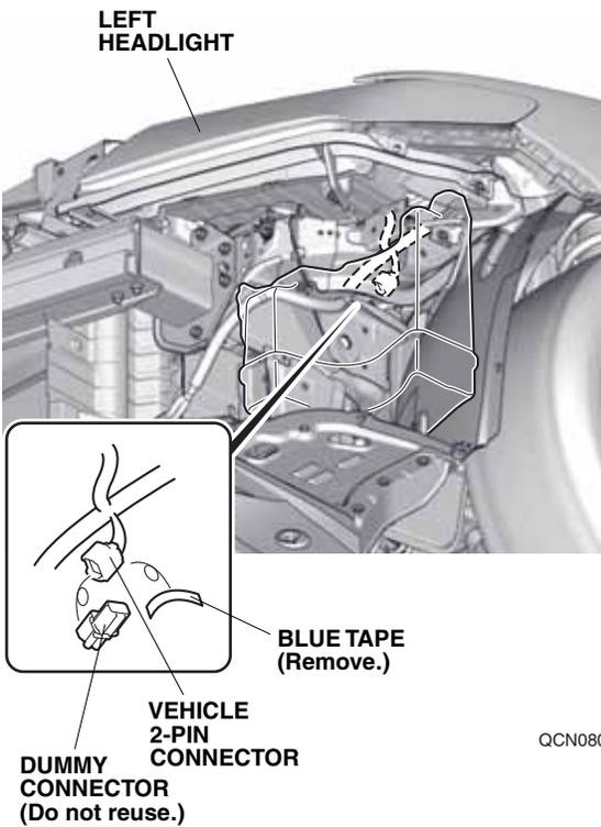
36. Install the wire tie with holder on the fog light subharness 2-pin connector.
