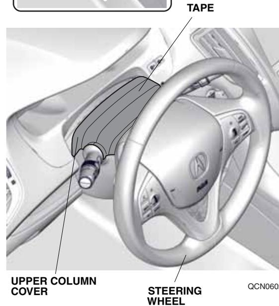
2. Press the engine switch to ON. Turn the steering wheel 90° counterclockwise. Using a plastic trim tool, release the upper column cover.
