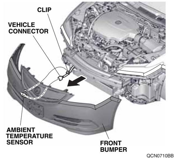
20. Remove the ambient temperature sensor.
