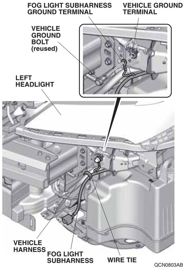
40. Secure the fog light subharness to the vehicle harness with one wire tie.
