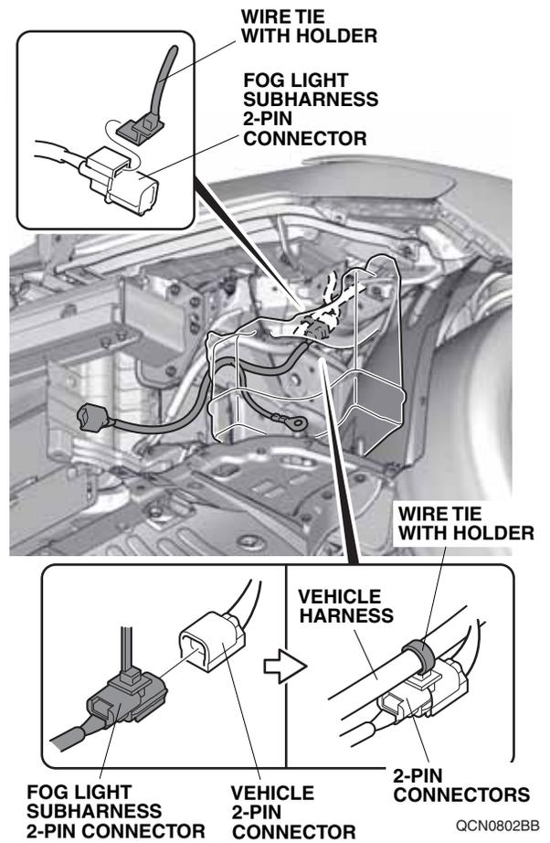
37. Plug the fog light subharness 2-pin connector into the vehicle 2-pin connector.
